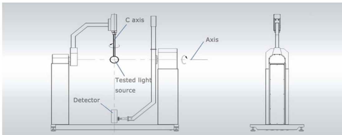
Figure Measurement Principle
