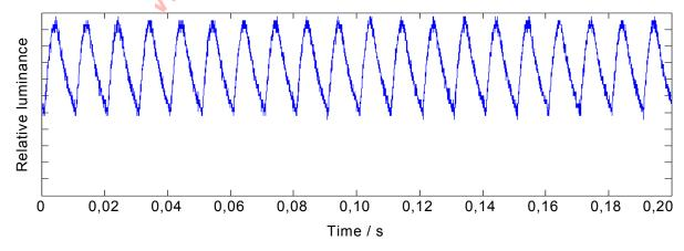
Figure 1 – Example of a time-modulated light output (unintended light modulation over time caused by AC mains)
