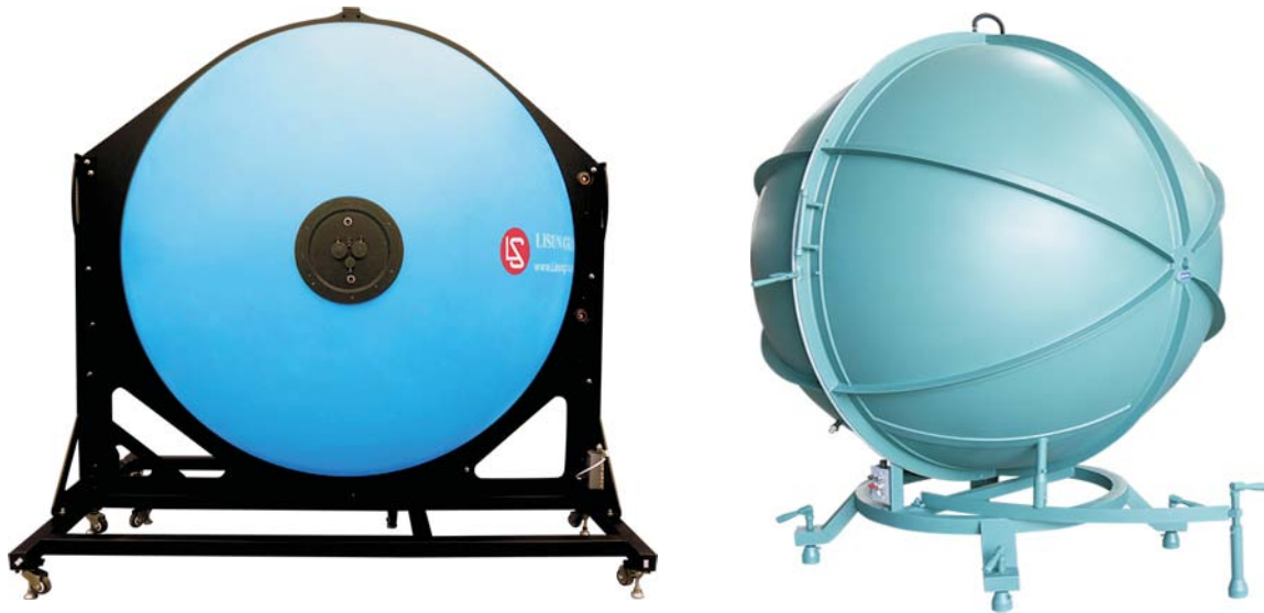
Figure: A Molding Integrating Sphere VS the traditional Integrating Sphere
